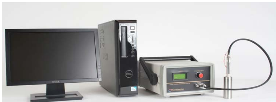
Shown are the controller connected to the platinum-wire sensor with the sensor residing in the sampling cell, along with the liquid specimen. For non-ambient temperature readings, the sampling cell inserts into a temperature control peripheral (not shown). The computer downloads data from the controller for storage and for the creation of spreadsheets and reports.
